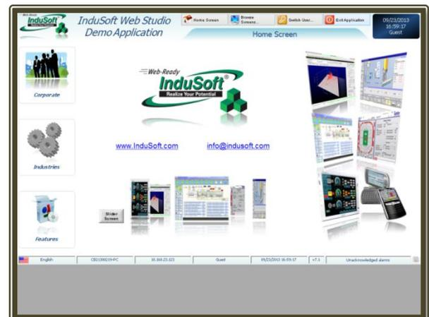
Figure 3: The InduSoft “PC Demo” application is natively built in 1280x800 resolution (5:3 or 1.6 aspect ratio). It is shown displayed on a 1366x768 monitor (16:9 or 1.67 aspect ratio) on the left, and a 1024x768 monitor (4:3 or 1.3 aspect ratio) on the right. The application is Auto-scaled to fit maximized in the monitor at either the Y-Max (left picture) leaving extra X space on the monitor, or X-Max (right picture) leaving extra Y space on the monitor.
