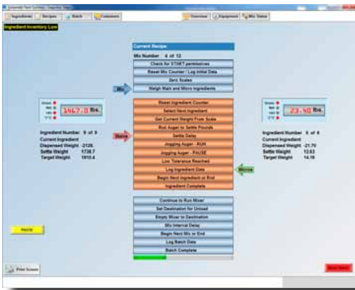
Figure 3: The user can monitor the status of the batch sequence. Animated arrows are used to point to the step(s) currently in progress. Many batches can take a few hours to complete. Instead of constantly checking on the status, a “Batch Complete” text message is sent to notify the user.
