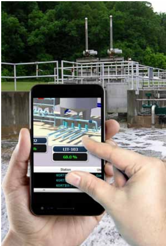
Figure 2: Multi-touch for HMI enables users to quickly access data and execute commands by using familiar gestures, such as pinch and swipe.
