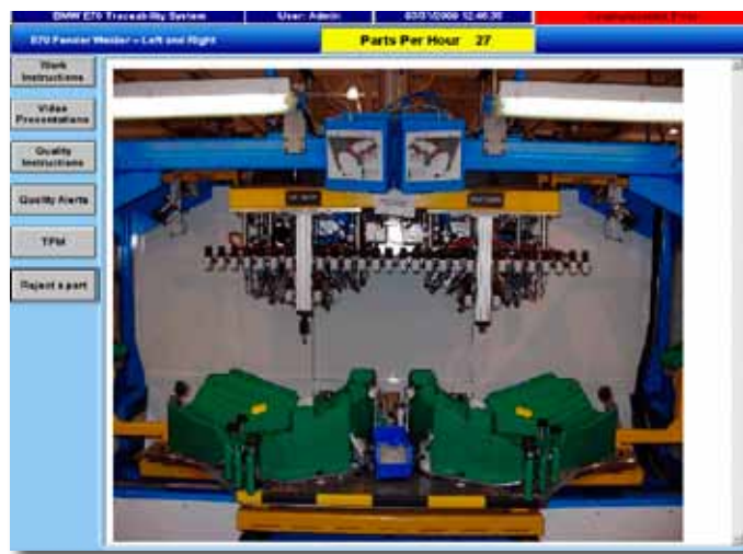
Figure 2: This fender welder is controlled by an Allen-Bradley PLC that reports to the InduSoft Web Studio software.
