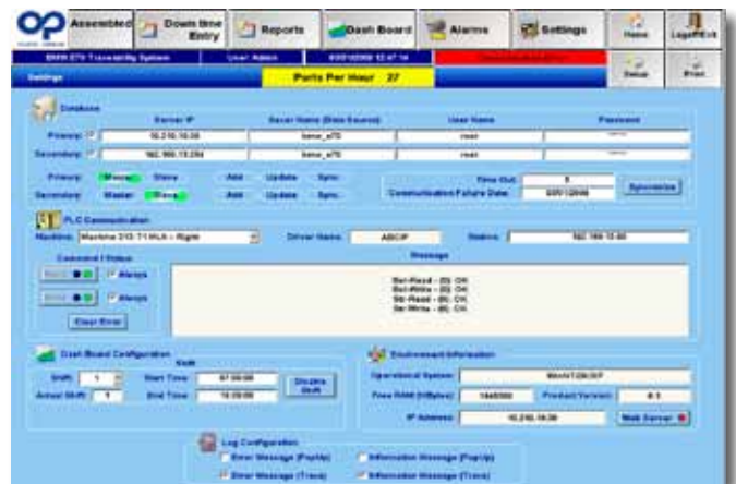
Figure 4: A settings screen shows how each PLC connects to InduSoft Web Studio.
