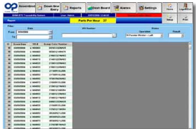
Figure 3: Summary screen lists fender modules by VIN, scoop color and the number of fenders made on a shift.
