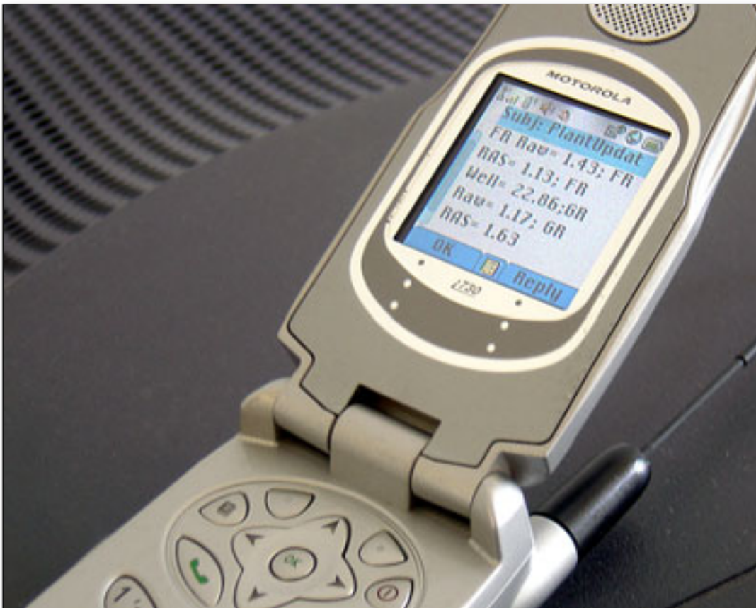
Smallest SCADA display ever! Status of the Xenia waste water treatment facility can be checked on the cell phones of duty personnel who are off-site.
